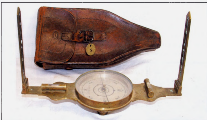
Brass circumferentor bearing the signature of Charles Potter, ca. 1870 that is on loan to the Educational Foundation from the AOLS Archives Committee. See the article in the Educational Foundation News on page 14.
